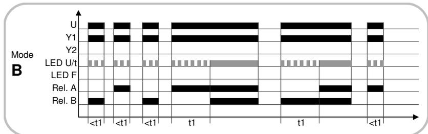
The highest priority is on the input for parallel operation (link Y2-Y3). If activated it will cause operation of both outputs anyway, with the fixed offset delay  $t_2$  only. The error indication on the unit will be illuminated if this input is active, unless there is a signal for the operation request input (Y1-Y2). (A defect sensor is assumed in this case) The input parallel operation (Y2-Y3) activated when the unit is set up for mode B will cause an error indication in any case.
