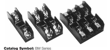
Type M Supplementary Fuseblocks For use with any  $1\frac{3}{32}$  ×  $1\frac{1}{2}$  Fuses (Bussmann KTK, FNQ, FNM, BAF, BAN and AGU) Ampere Rating:  $\frac{1}{10}$  to 30A
