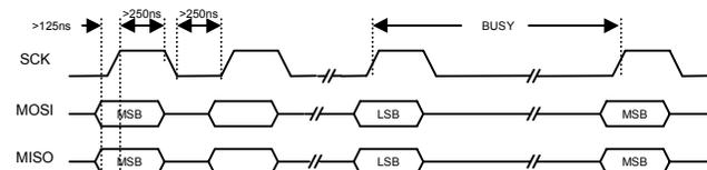
Fig2: Waveforms show TTL synchronous serial.
