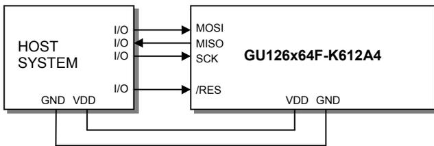
When using synchronous communications. Data is clocked in on the rising edge of SCK. The most significant bit of the data byte should be sent first.
