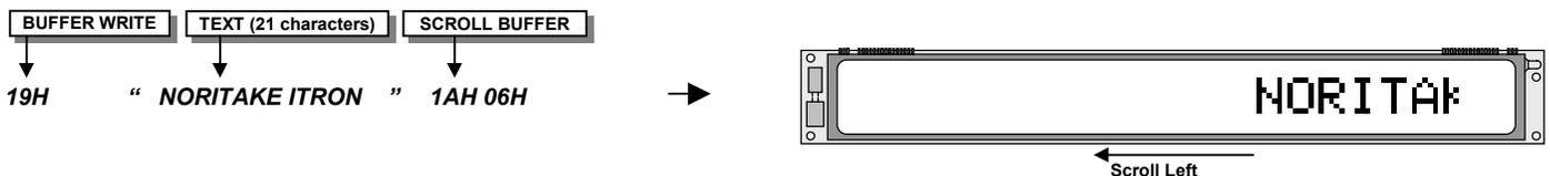
Using the 'Write Mode' command, the user can scroll longer text messages. Each character written to the display will scroll on from either the right or left side (depending upon the 'Write Direction').
