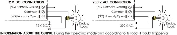
INFORMATION ABOUT THE OUTPUT. During the fluctuation or an incorrect working of the output. In such case, you have to install an anti-spark circuit between both contacts of the used relay, as it is indicated on the schedule.
