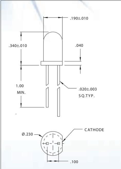
The CMD505X series of industry standard LED lamps is produced with GaAsP. This standard red light source LED is available with various lens effects for backlighting and direct viewing applications. This compact, rugged and lightweight LED requires low power and allows for versatile mounting on a PC board or panel.
