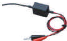
Differential voltage probe
