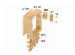
Larger housing are easily assembled: the intermediate plate (ZP) and the connection spigot (VZ) enable 2 or more housing to be mechanically joined together. The ZP joins together the housing frames in the area of the clamping yoke unit and the VZ the housing frames at the bottom of the frame. The fixing in combination foot or the mounting plate allows the housing to be mounted on the rail or directly.
