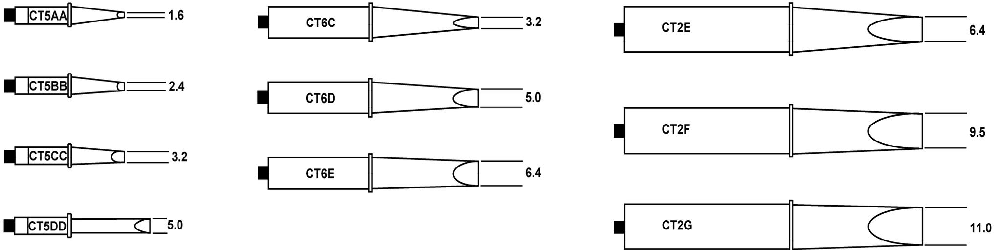
Note: Add 6,7,8,9 to the rear part of the Part No for temp rating (6= 325C, 7= 375C, 8= 425C, 9= 475C)
