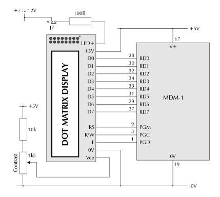
$^\ast$  Some character dot matrix display feature a single row of 16 connections, though the same pin functions are brought out.
