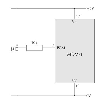
You can use the RB3/PGM port to mimic/simulate an input from a peripherals such as a switch, alarm trigger etc.
