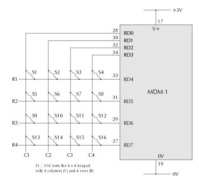
You can add an external matrix keypad to the RD port. The keypad can be up to  $4 \times 4$  buttons in size. A keypad decoder routine is supplied with MDM-DEV-1 and is available for download from the Lascar website.
