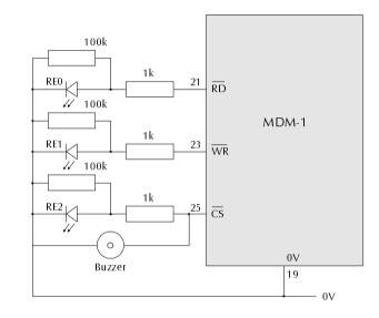
You can use the LEDs on the 3-bit RC port to indicate/mimic/simulate peripherals such as relays, annunciators, status of controlled equipment etc. In addition, the buzzer on Port RE2 can be used as an alarm indicator.
