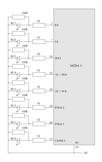
You can use the LEDs on the 8-bit RC port to indicate/mimic/simulate peripherals such as relays, annunciators, status of controlled equipment etc.
