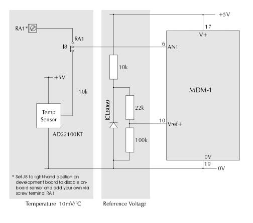
A range of linear voltage-output temperature sensors can be used with MDM-DEV-1 (e.g. LM35xx, AD 22100xx, etc.). Note however that the module may require new calibration values in software if a sensor with an output voltage of other than 22.5mv/°C is used.
