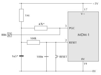
\* Not strictly part of the reset circuit, hold RESET down for 2 seconds or more to enable the PIC's in-circuit debugger pin PGC.
