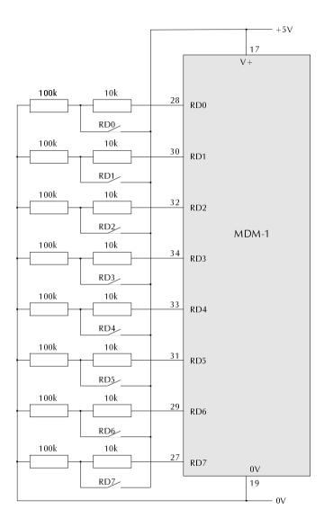
You can use the switches on the 8-bit RD port to mimic/simulate inputs from peripherals such as switches, alarm triggers etc.
