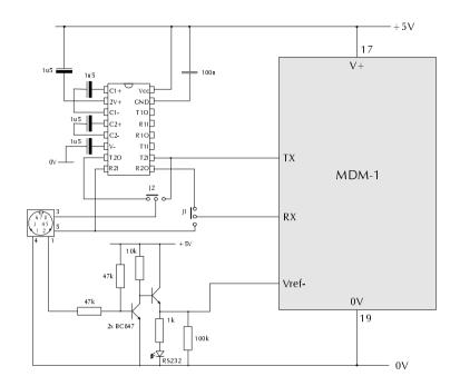
The development board features a complete RS232 conversion circuit, which accepts inputs from the Rx and Tx ports on the MDM-1, and allows the module to communicate with the outside world. Switching over J1 and J2 will bring out the MDM's Rx and Tx ports, which can then be used to interface to other communication protocols (e.g. RS485).
