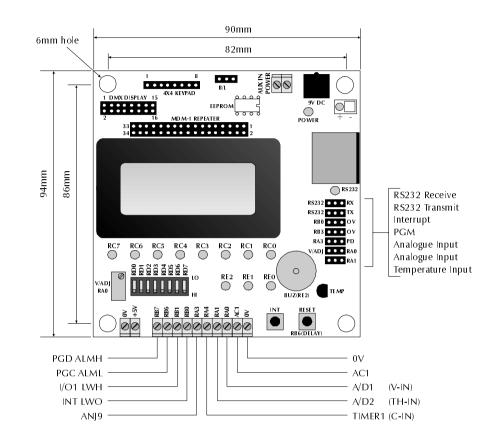
Component lay-out and dimensions of the Development Board.
