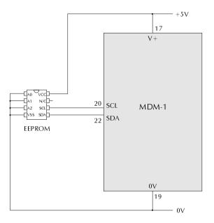
You can solder an optional EEPROM device (not supplied) into the MDM-DEV-1 PCB. The use of an IC-socket is advised. Take care to insert the socket on the top of the PCB, and ensure that pin 1 is correctly located. The EEPROM footprint and pin-out are compatible with a variety of serial EEPROM families and memory sizes (e.g. Microchip 24LC65, 24AA65).
