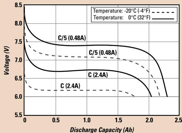
Voltage and capacity of DURACELL DR30 Ni-MH batteries at various discharge temperatures and rates.
