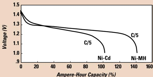
Comparison of discharge voltage and capacity of same-size Ni-MH and Ni-Cd cells.
