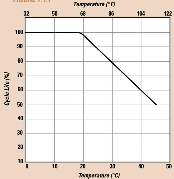
Impact on cycle life from repeated charging and discharging at various ambient temperatures.
