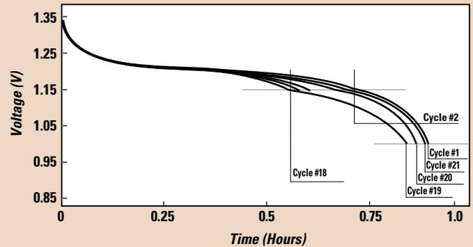
Effects on Ni-MH cell capacity due to repetitive partial discharges.
