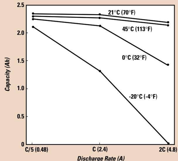
Typical capacity of DURACELL DR30 batteries under constant current discharges at various temperatures. [Conditions: Charge: 1C to  $-\Delta V = 60\text{mV}$  @ 21°C (70°F); Discharge to 6.0V]
