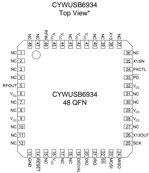
Figure 8-2. CYWUSB6934, 48 QFN – Top View
