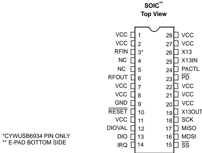
Figure 8-1. CYWUSB6932/CYWUSB6934, 28 SOIC – Top View
