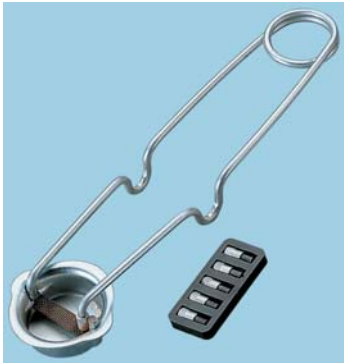
Suitable for igniting LP Gas torches. Cup shaped shield traps the gas and assures ignition.
