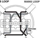
TO SWITCH TO LIGHT SWITCHED LIVE WIRE (BLUE) MUST HAVE BROWN SLEEVE
