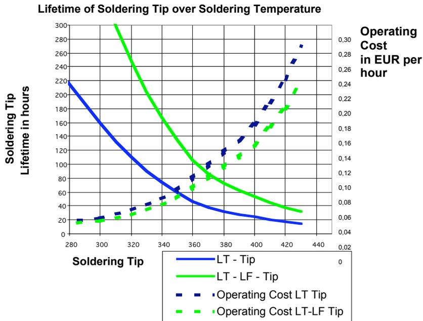
The graph shows that the LT-LF Soldering-Tips provide a cost reduction and the main influence of lifetime is the soldering temperature.
