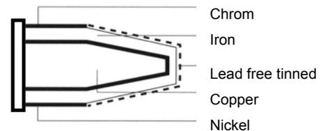
For the ability of excellent thermal conductivity, a soldering tip consists of a Copper core. I.e. Silver would be better, but is much more expensive.
