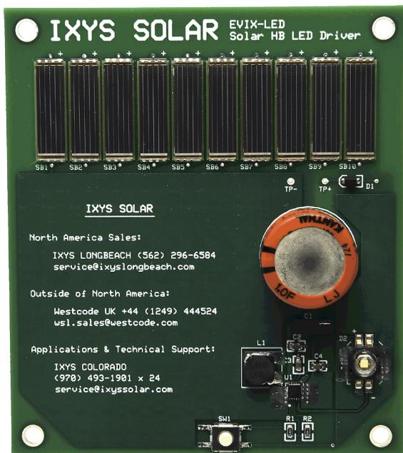
Ten series-connected SolarBITS convert sunlight to a current that charges a supercapacitor to 5V. A buck/boost converter uses the energy stored in the supercap to drive the LED with a constant current of 1A for several seconds, even as the voltage across the supercap decreases below the LED's forward voltage requirement.
