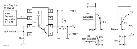
Figure 1. Switching Test Circuit
