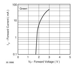
Figure 10. Forward Current vs. Forward Voltage
