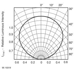
Figure 4. Rel. Luminous Intensity vs. Angular Displacement
