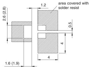
Dimensions: IR and Vaporphase (Wave Soldering)
