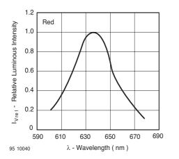
Figure 9. Relative Intensity vs. Wavelength
