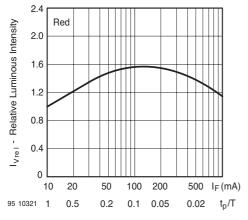
Figure 7. Rel. Lumin. Intensity vs. Forw. Current/Duty Cycle
