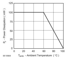
Figure 1. Power Dissipation vs. Ambient Temperature
