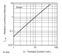
Figure 13. Relative Luminous Intensity vs. Forward Current
