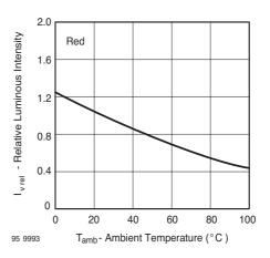
Figure 6. Rel. Luminous Intensity vs. Ambient Temperature
