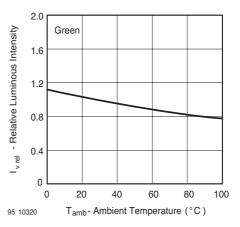
Figure 11. Rel. Luminous Intensity vs. Ambient Temperature
