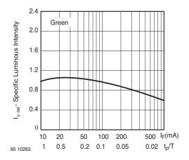
Figure 12. Specific Luminous Intensity vs. Forward Current
