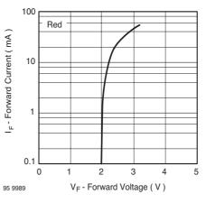
Figure 5. Forward Current vs. Forward Voltage
