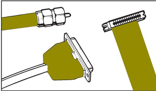
3M™ Shielding Tapes are used as ground planes or shields for electronic cables and connectors. The tape is bonded to the cable's conductive sheath and to the metallic lip of the connector to provide a complete shield from end to end.
