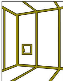
Shielding tapes provide effective, economical shielding of seams and apertures in shielded rooms.
