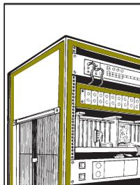
3M shielding tapes provide a reliable, durable contact surface for conductive gaskets for EMI shielding of the doors and panels of electronic cabinets and enclosures.
