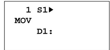
Program data registers D10 and D50 for source operand S1 and destination operand D1. The cursor can be moved using the and keys.
