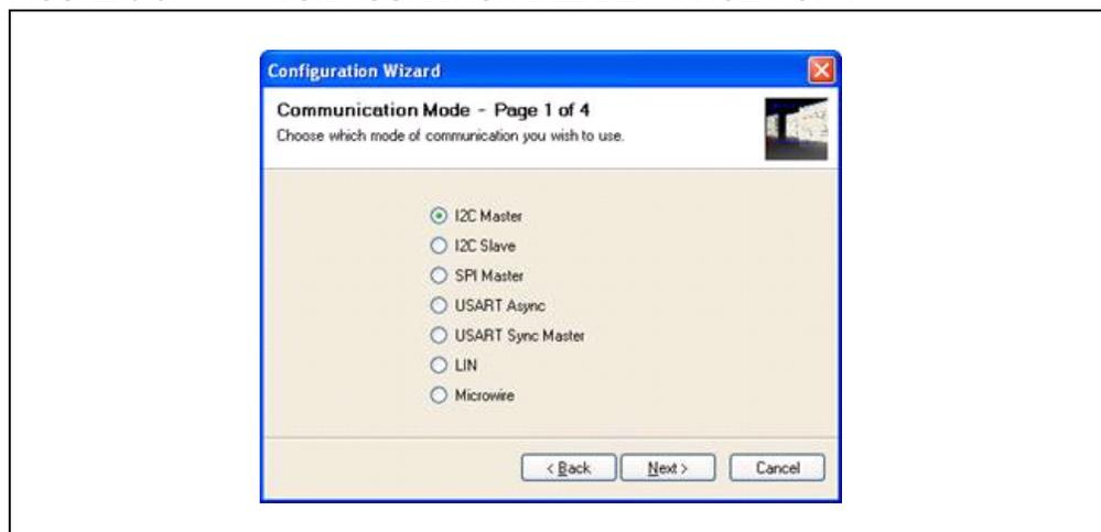
In this example, I<sup>2</sup>C Master Communication's mode is selected. The Configuration Wizard Page 2 of 4, as shown in Figure 3-4, allows you to select the bus speed. A more comprehensive list of bus speeds can be chosen from the Configuration Window by selecting *PICKit Serial Analyzer > Configure Communications Mode* from the menu bar.
