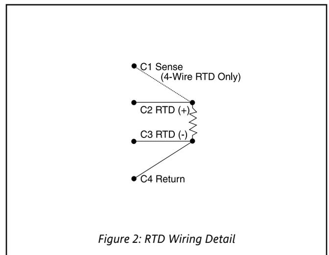
Figure 2: RTD Wiring Detail
