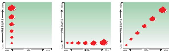
Time pressure dispensing is the most common dispensing method used today. Its popularity stems from the need for process control and the fact it is possible to dispense from disposable containers without the need for cleaning.
