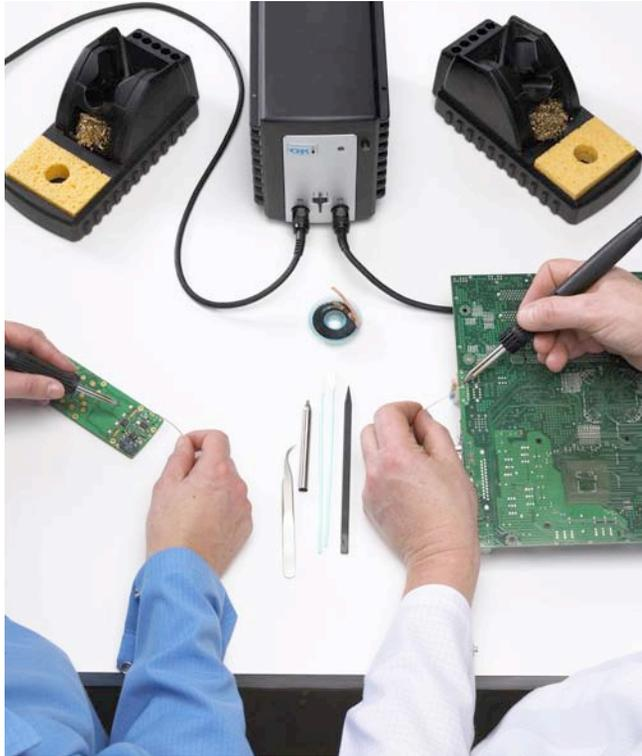
The MFR-2200 Series features dual output capability allowing users to select operation of one hand-piece or two hand-pieces **simultaneously**.
