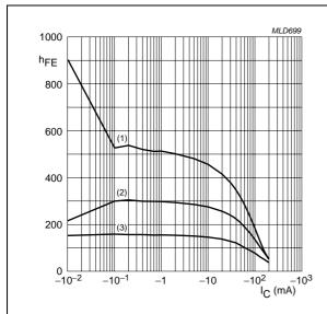
**TR2 (PNP)**;  $V_{CE} = -5 \text{ V}$ .
