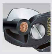
Cut effected with a Cable Shear: easy, clean cut without any deformation of the cable
