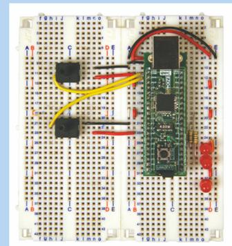
When you are happy with your design click one button to send the program directly to the ECIO device. Remove the USB lead and press the reset button and your program starts to run.
