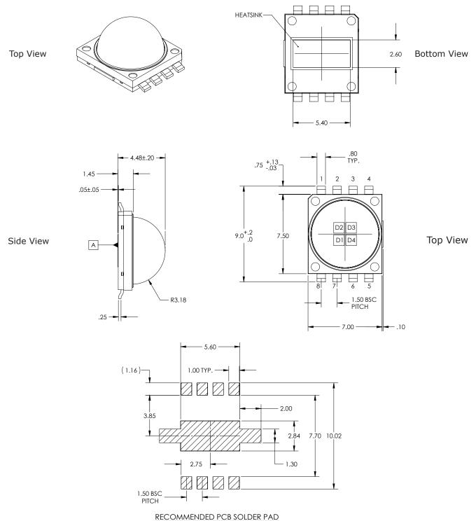
Tolerances: ±.10 Solder mask windows must be .05 mm bigger than PCB Solder Pad.
