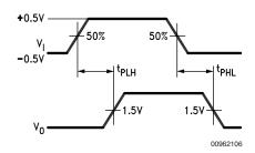
Amplitude: 1.0V Offset: 0.5V Pulse Width: 100 ns PRR: 5.0 MHz  $t_r = t_f \leq 5.0 \text{ ns}$
