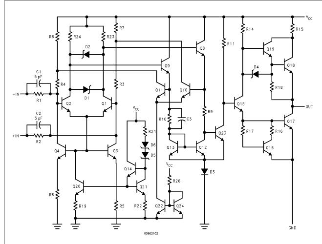
FIGURE 1. Equivalent Circuit
