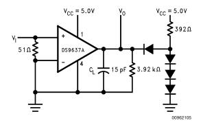
$\mathbf{C}_{\mathsf{L}}$  includes jig and probe capacitance. All diodes are FD700 or equivalent.
