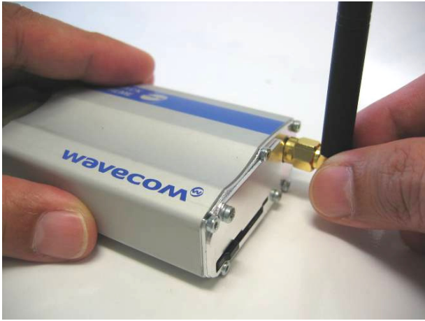
Attach the GSM antenna
