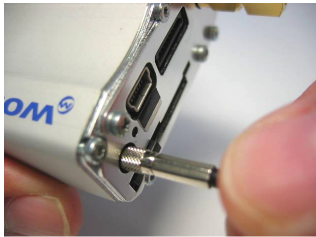
Connect the GPS antenna cable
