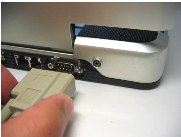
Connect the serial cable other end to PC COM Port
