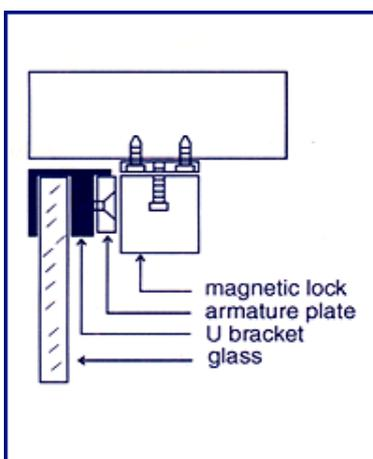
**Note:** This aluminium fabricated bracket is suitable for 10mm to 12mm glass doors. Before the installation takes place, ensure the glass meets the thickness requirement. After confirming the glass size is correct apply glue to the glass area as required then tighten the three screws provided, also apply a small amount of glue to the armature screw in order to prevent it becoming loose, then fix the armature plate remembering to fit
