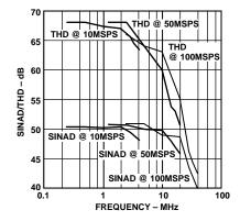
Figure 3. SINAD/THD vs.  $f_{OUT}$  (AVDD and DVDD = 5.0 V)
