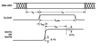
Figure 1. Timing Diagram
