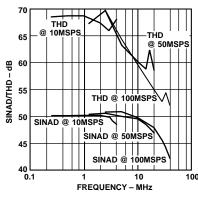
Figure 7. SINAD/THD vs.  $f_{OUT}$  (Differential Output, AVDD and DVDD = 3.0 V)
