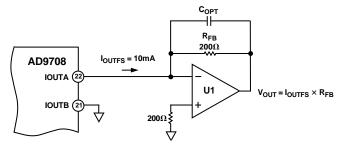
Figure 17. Unipolar Buffered Voltage Output
