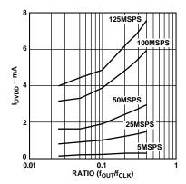
Figure 21.  $I_{DVDD}$  vs. Ratio @ DVDD = 3 V
