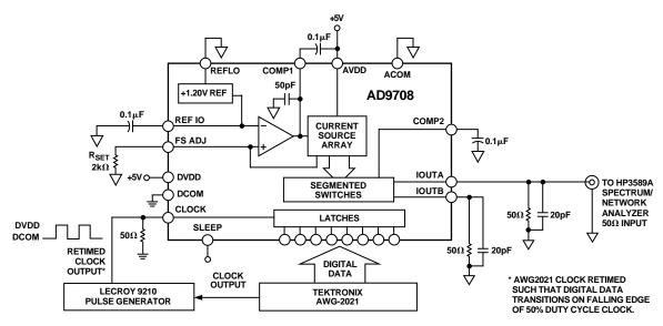
Figure 2. Basic AC Characterization Test Setup
