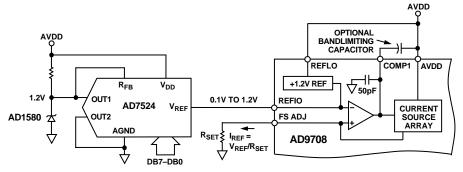
Figure 15. Single-Supply Gain Control Circuit
