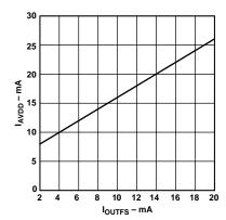
Figure 19. I<sub>AVDD</sub> vs. I<sub>OUTFS</sub>
