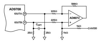
Figure 25. Single-Supply DC Differential Coupled Circuit
