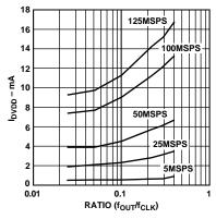
Figure 20.  $I_{DVDD}$  vs. Ratio @ DVDD = 5 V
