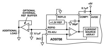
Figure 13. Internal Reference Configuration
