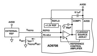
Figure 14. External Reference Configuration
