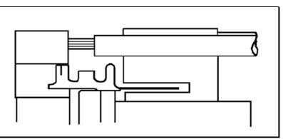
9. Hold the cable steady and fully compress the handle, to complete the crimping operation. Do not attempt to open the tool before fully compressing it, as this may damage both tool and crimp.
