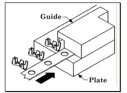
7. Push the contact until the contact touches the stopper-block. Check that the carrier of the contact goes into the groove of the carrier-cutter.
