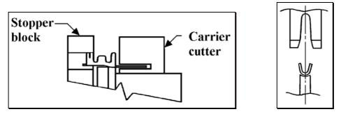
8. Compress the hand tool by one notch, then position the cable within the tool as shown below.
