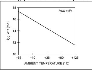
Standby Supply Current vs. Ambient Temperature
