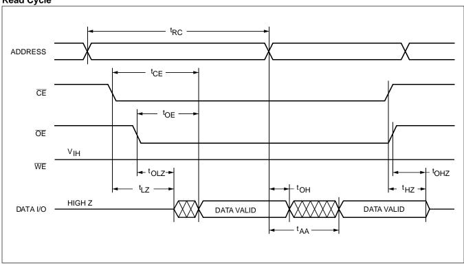
Notes: (3)  $t_{LZ}$  min., $t_{HZ}$ ,  $t_{OLZ}$  min., and  $t_{OHZ}$  are periodically sampled and not 100% tested.  $t_{HZ}$  max. and  $t_{OHZ}$  max. are measured, with  $C_L$  = 5pF, from the point when  $\overline{CE}$  or  $\overline{OE}$  return HIGH (whichever occurs first) to the time when the outputs are no longer driven.
