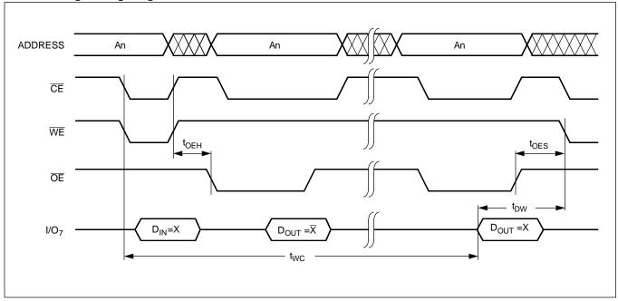
**Toggle Bit Timing Diagram**
