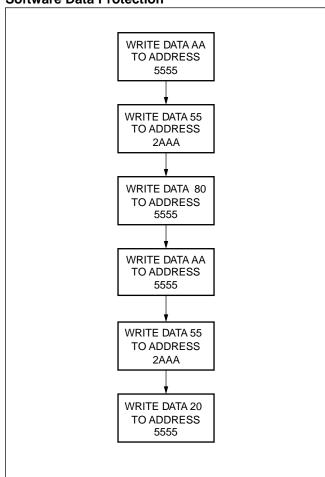
In the event the user wants to deactivate the software data protection feature for testing or reprogramming in an E²PROM programmer, the following six step algorithm will reset the internal protection circuit. After  $t_{WC}$ , the X28C010 will be in standard operating mode.
