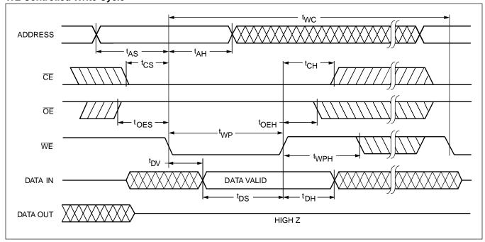
**Notes:** (4) t<sub>wc</sub> is the minimum cycle time to be allowed from the system perspective unless polling techniques are used. It is the maximum time the device requires to complete internal write operation.
