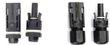
H4 with 4mm contact with 2,5sqmm solar wire Current rating: 90A, 56A TUV, 35A UL
