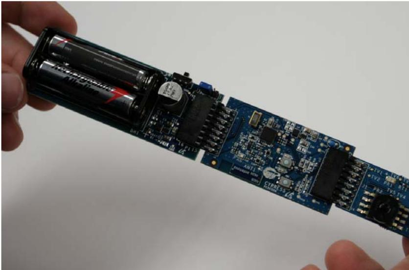
7. Switch on power to the RF Expansion Board by sliding the ON/OFF switch on the battery pack towards the RF Expansion Board.
