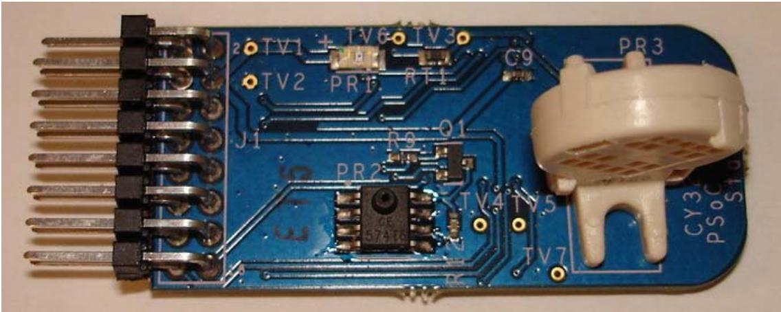
The Weather Station Expansion Board sends the sensor data over I<sup>2</sup>C to the RF Expansion Card, which is contained in the CY3271 PSoC FirstTouch Start Kit.
