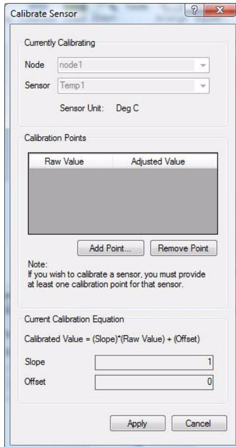
Open this dialog using the **Tools > Selected Sensor > Calibrate** menu item and **Calibrate Sensor** toolbar button. Use the buttons **Add Point** and **Remove Point** to add or remove calibration data pairs.
