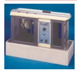
A vertical etching machine with a clean spray working process for continuous etching and rinsing. The spray nozzles, with flat spray, are arranged at both sides of the board. The boards are transported through the machine by non marking rotating wheels. The housing is fully constructed of non-corrosive welded PVC
