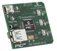
The USB Starter Kit II has the same form factor and expansion connector as other PIC32 Starter Kits.
