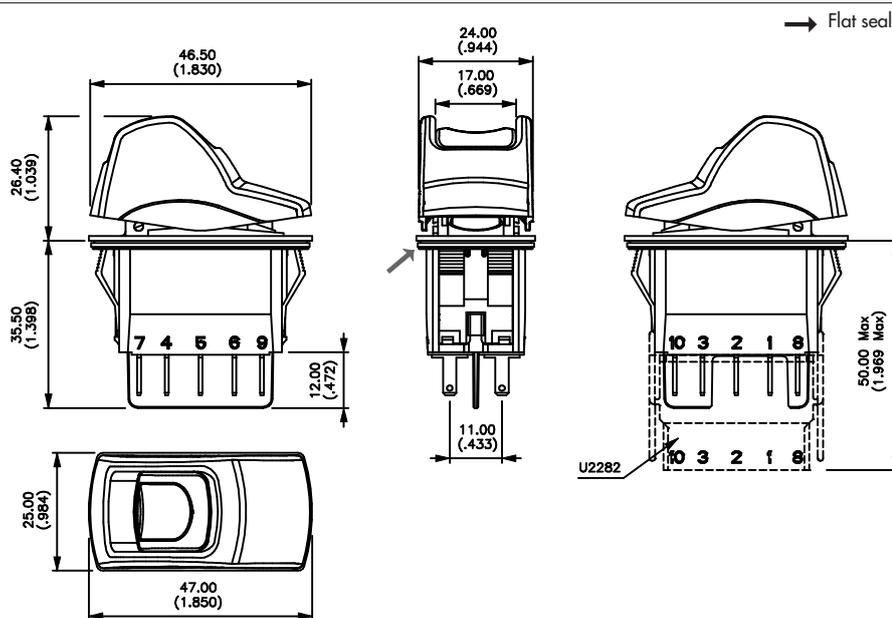
**Dimensions :** First dimensions are in mm while inches are shown as bracketed numbers.
