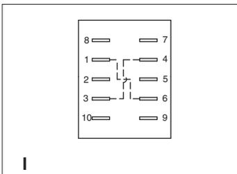
To have a polarity inversion (typical application : fan motor).
