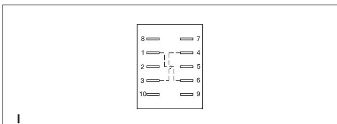
Power supply between 2 and 5 - Load between 1 and 4 or 3 and 6. Available with H and J quick-connect terminals.
