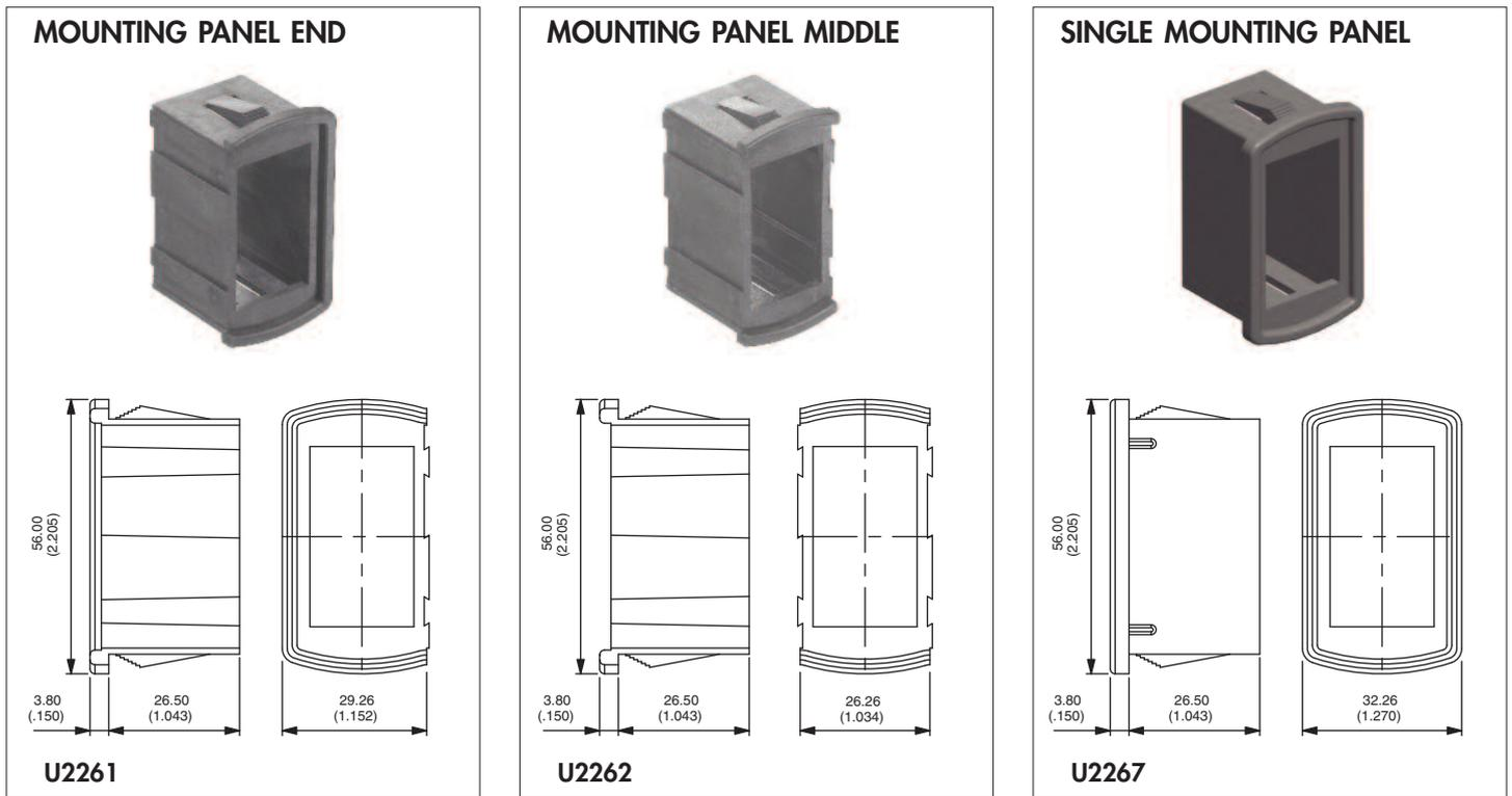
Recommended panel thickness : 1,10 mm - 1,80 mm - 2,60 mm - 3,40 mm - 4,20 mm - 5 mm - 5,80 mm
