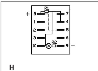
To obtain 2 symbol illumination levels (night illumination when OFF and higher illumination when ON).
