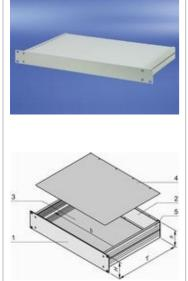
h = clear height (overall) (H -8.1 mm) b = clear installation width = 403 mm
