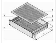
h = clear height (overall) (H -8.1) b = clear installation width = 403 mm
