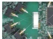
Using high speed optical fiber-based transmissions, the module achieves high speed ADC clock and data isolation.
