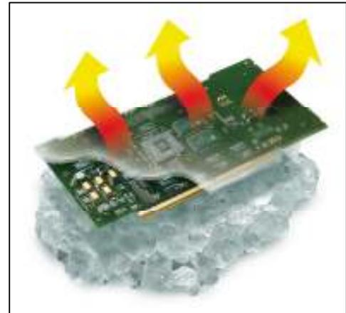
These transfer materials come in a wide variety of forms; liquid adhesives, pastes, gels, potting compounds, sheets, rolls, pads and sprays. They also utilise an equally large array of chemistries. Choice of material will be driven by a combination of factors including:
