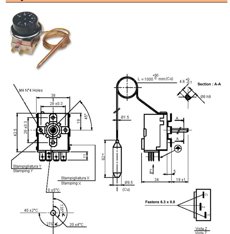
Switching point with thermostat at temperature =  $20^{\circ}$ C.
