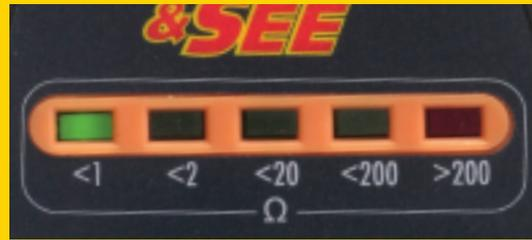
CLEAR LESS THAN 1M $\Omega$  LOOP TEST READING
