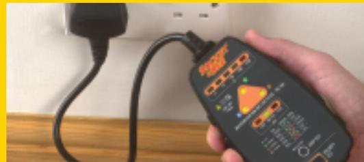
BUILT-IN SOCKET TEST FUNCTION AND CORRECT VOLTAGE RANGE DISPLAY
