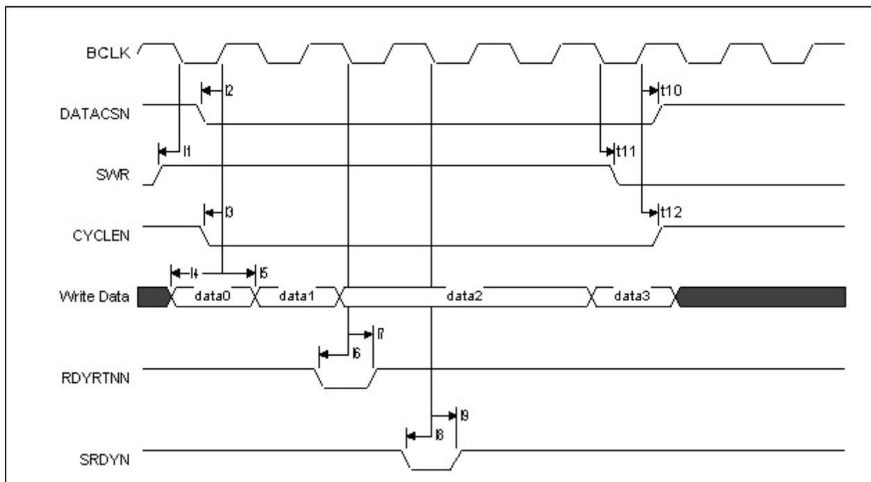
**Figure 16. Synchronous Burst Write Cycles – VLBUSN = 1**
