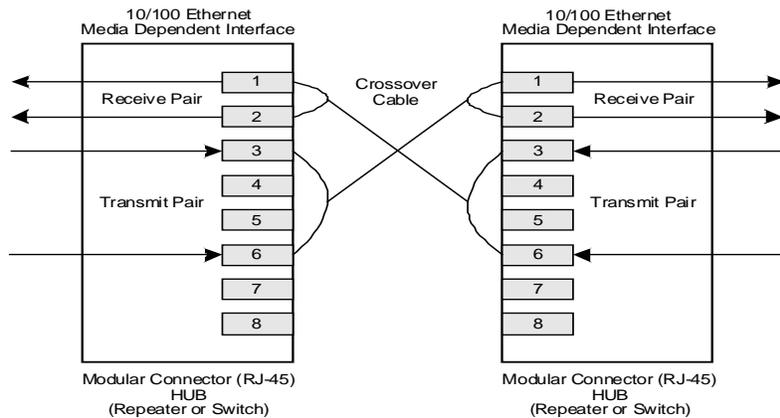
**Figure 7. Typical Crossover Cable Connection**
