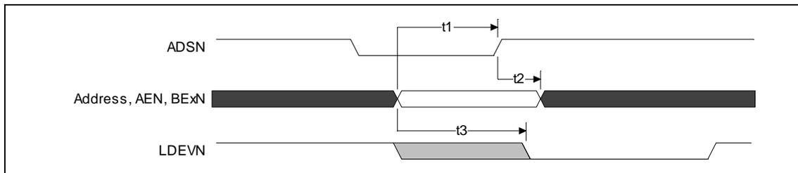
**Figure 15. Address Latching Cycle for All Modes**
