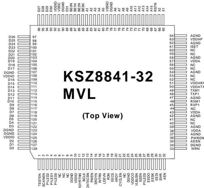
Figure 5. Option – KSZ8841-32 MVL 128-Pin PQFP (Top View)
