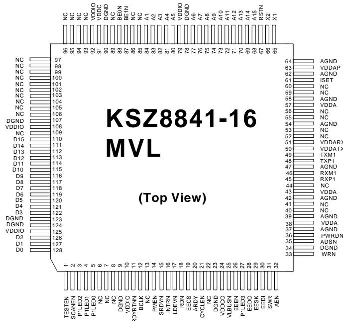
Figure 3. Option – KSZ8841-16 MVL 128-Pin PQFP (Top View)
