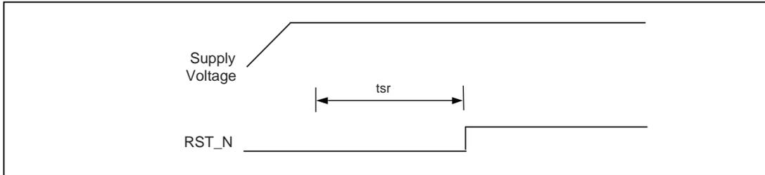
**Figure 21. Reset Timing**
