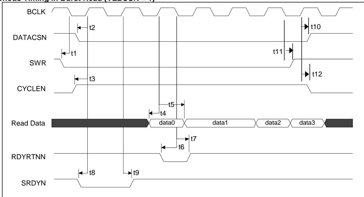
**Figure 17. Synchronous Burst Read Cycles – VLBUSN = 1**
