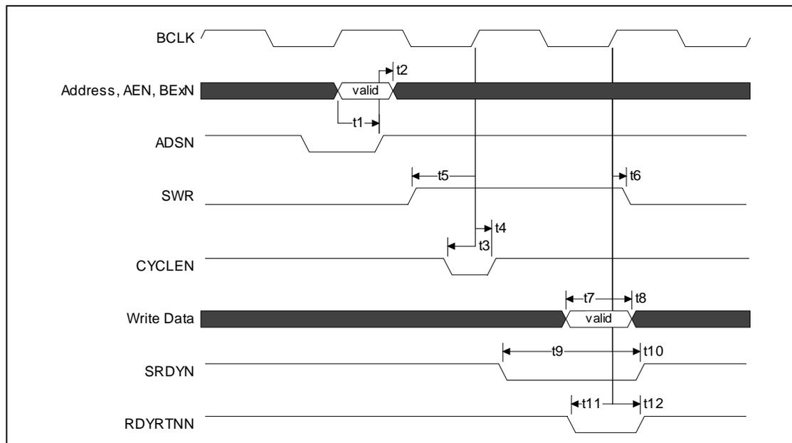
**Figure 18. Synchronous Write Cycle – VLBUSN = 0**
