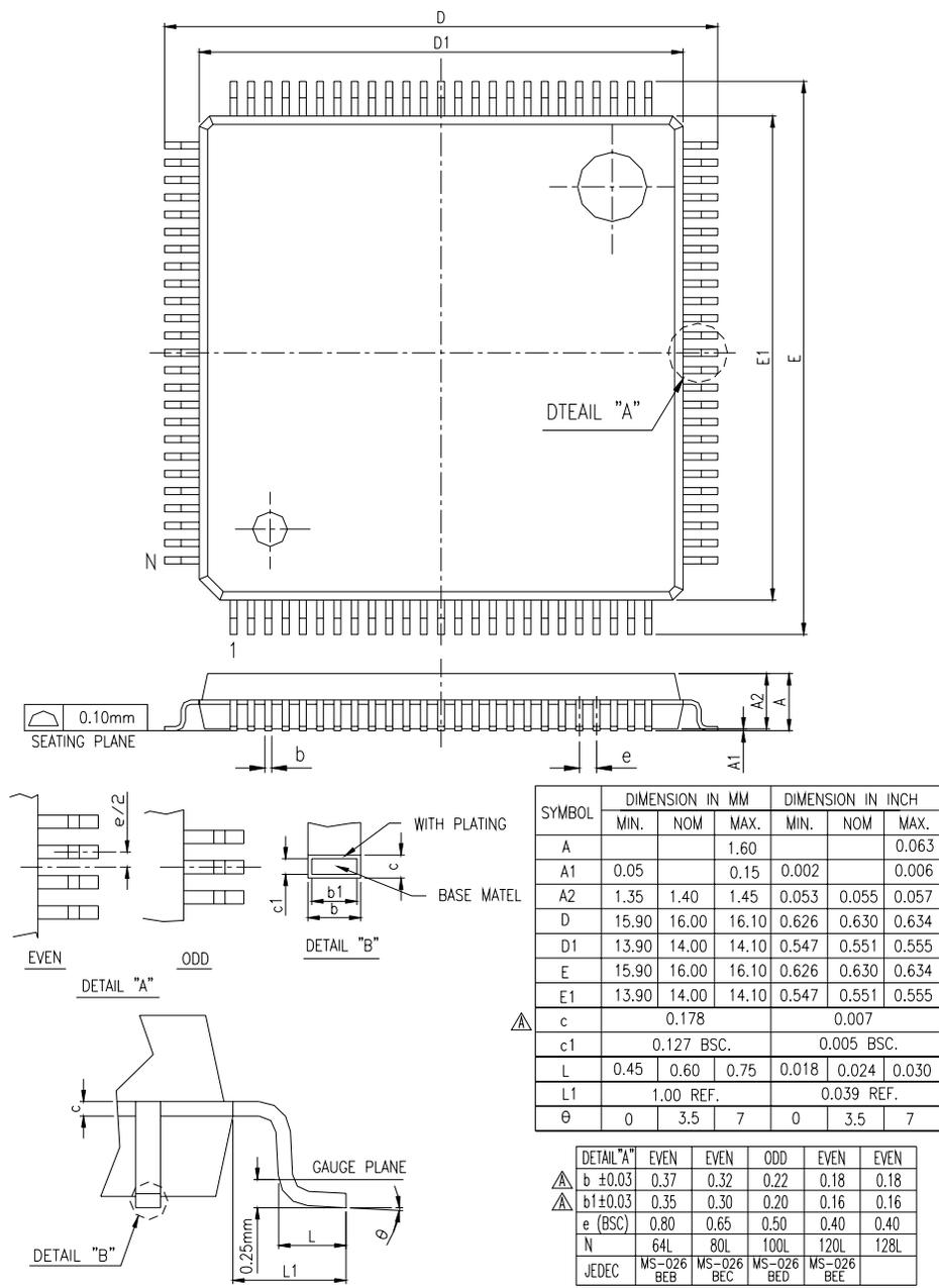
Figure 24. Optional 128-Pin LQFP Package
