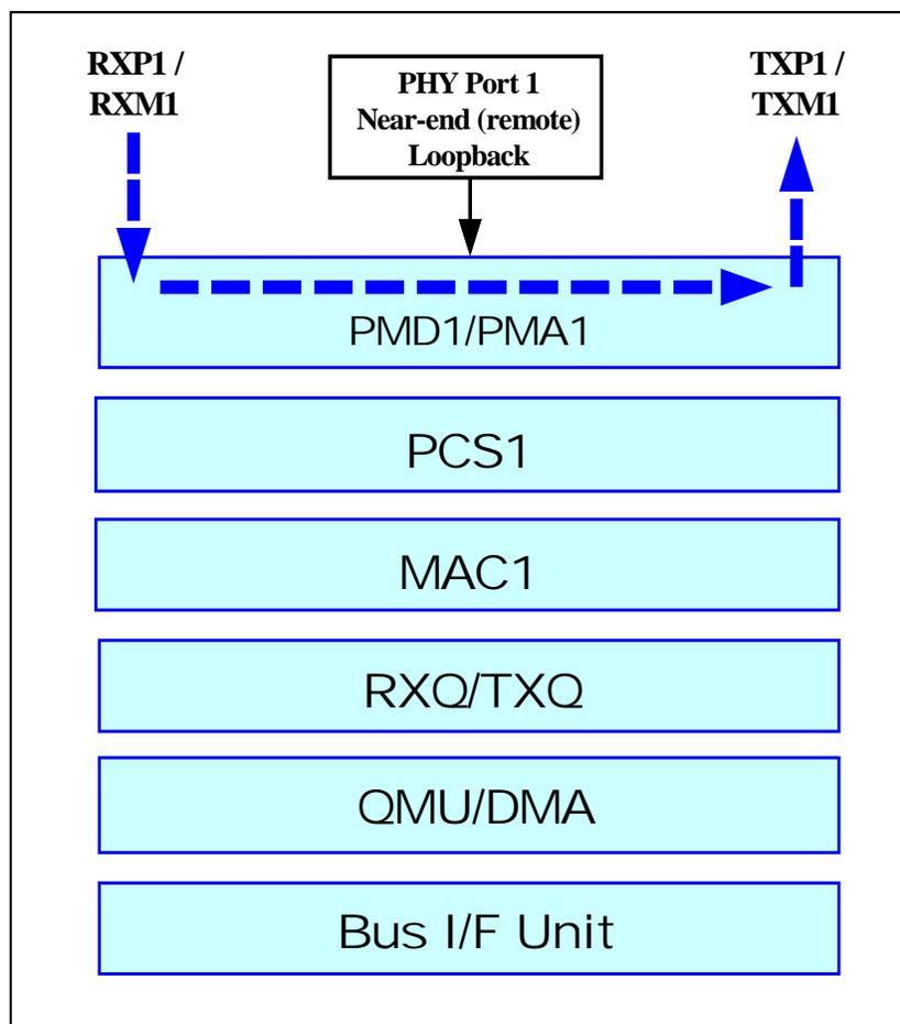
Figure 11. PHY Port 1 Near-end (Remote) Loopback Path
