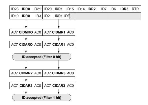
Figure 17-4. 16-bit Maskable Acceptance Filters
