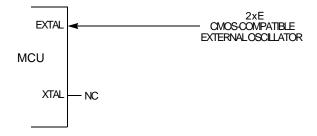
Figure 3-6. External Oscillator Connections
