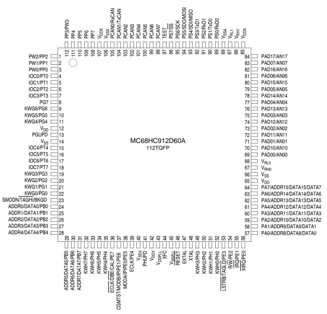
Note: TEST = This pin is used for factory test purposes. It is recommended that this pin is not connected in the application, but it may be bonded to 5.5 V max without issue. Never apply voltage higher than 5.5 V to this pin.
