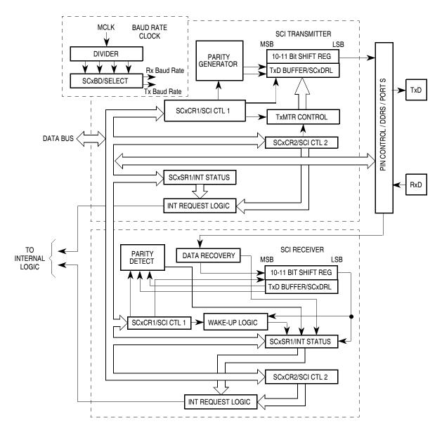
Figure 15-2. Serial Communications Interface Block Diagram
