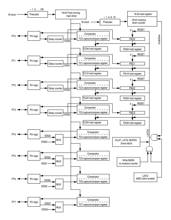
Figure 14-1. Timer Block Diagram in Latch Mode
