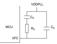
Figure 3-5. PLL Loop Filter Connections
