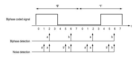
Figure 16-2. Biphase coding and error detection
