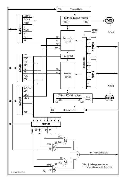
Figure 16-3. MI BUS Block Diagram
