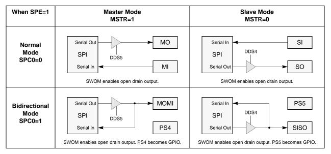
Figure 15-6. Normal Mode and Bidirectional Mode
