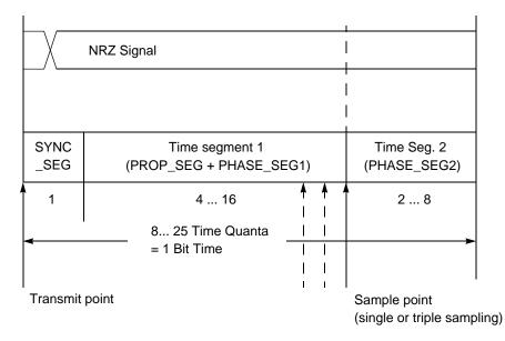
Figure 17-8. Segments within the Bit Time
