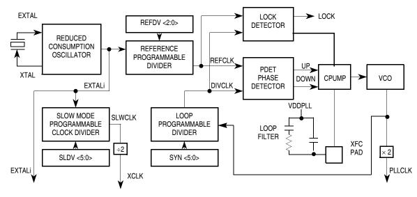
Figure 11-2. PLL Functional Diagram
