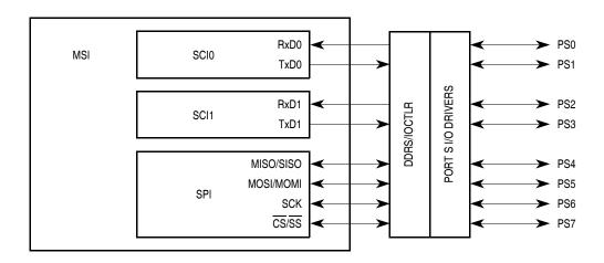
Figure 15-1. Multiple Serial Interface Block Diagram
