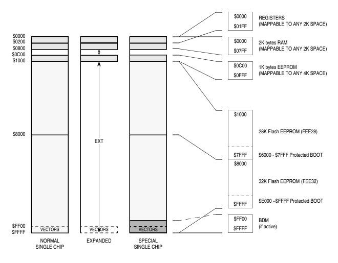
The following diagrams illustrate the memory map for each mode of operation <u>immediately after reset</u>.
