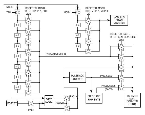
Figure 11-8. Clock Chain for ECT
