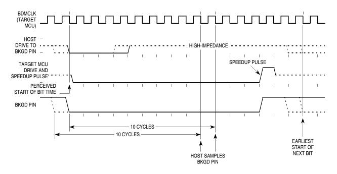
Figure 19-3. BDM Target to Host Serial Bit Timing (Logic 0)
