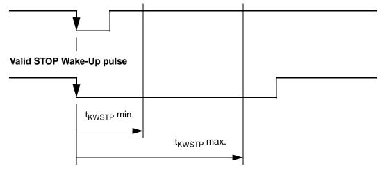
Minimum time interval between pulses to be recognized as single pulses
