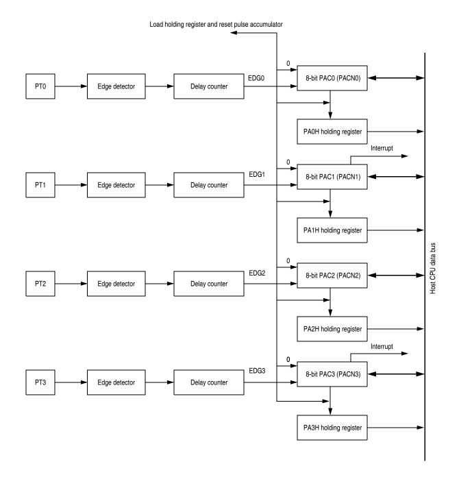
Figure 14-3. 8-Bit Pulse Accumulators Block Diagram
