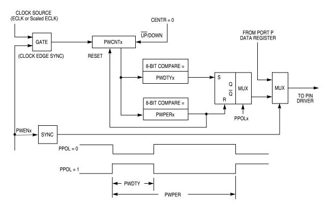
Figure 13-1. Block Diagram of PWM Left-Aligned Output Channel
