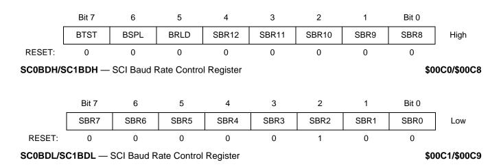
SCxBDH and SCxBDL are considered together as a 16-bit baud rate control register.
