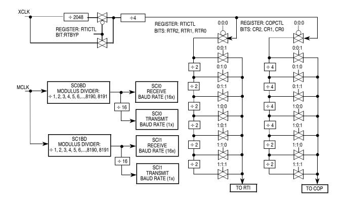
Figure 11-7. Clock Chain for SCI0, SCI1, RTI, COP
