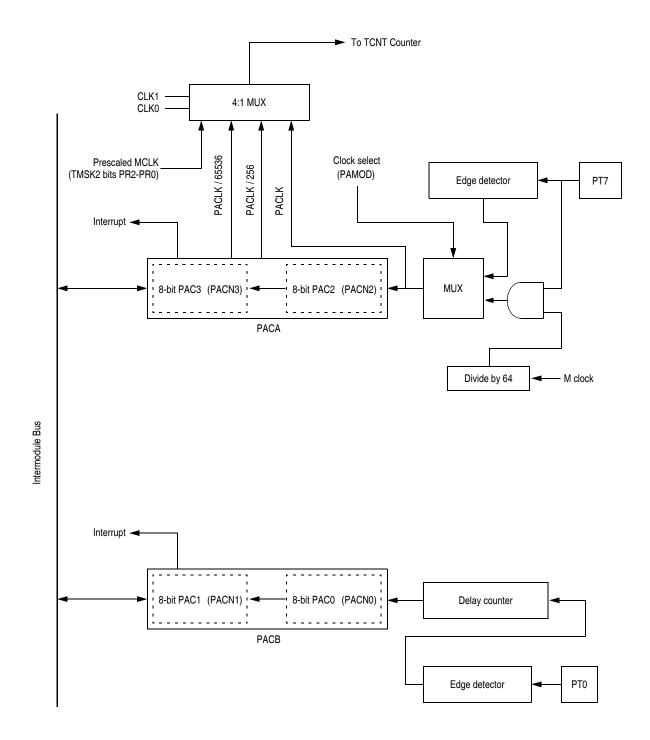
Figure 14-4. 16-Bit Pulse Accumulators Block Diagram
