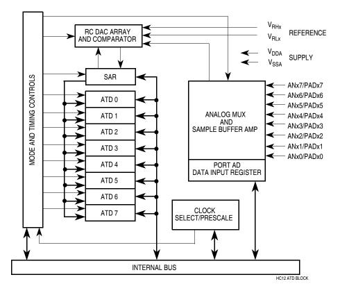
Figure 18-1. Analog-to-Digital Converter Block Diagram
