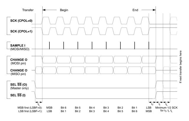
Figure 15-5. SPI Clock Format 1 (CPHA = 1)
