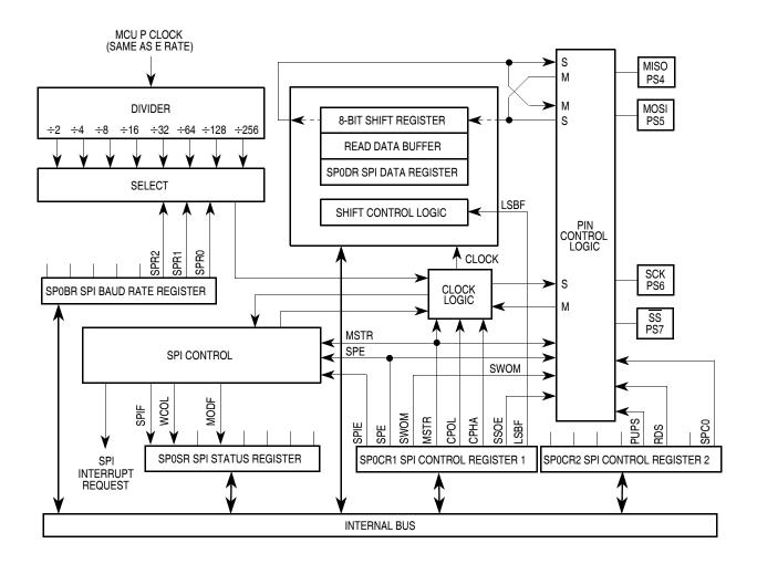
Figure 15-3. Serial Peripheral Interface Block Diagram
