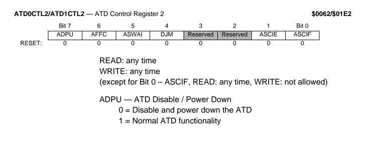
This bit provides program on/off control over the ATD module allowing reduced MCU power consumption when the ATD is not being used. When reset to zero, the ADPU bit aborts any conversion sequence in progress. Because the analog electronics is turned off when powered down, the ATD requires a recovery time period when ADPU bit is enabled.
