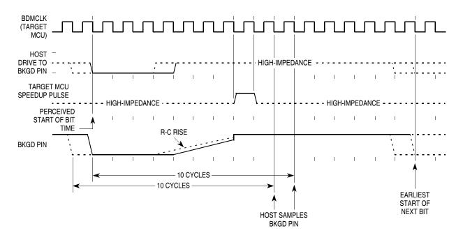
Figure 19-2. BDM Target to Host Serial Bit Timing (Logic 1)
