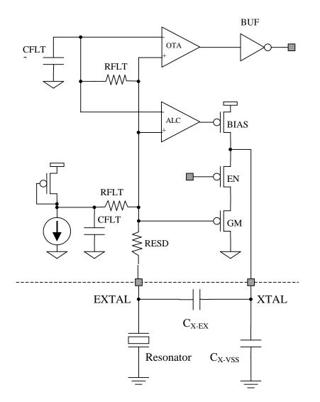
Figure 12-1. MC68HC912D60A Colpitts Oscillator Architecture
