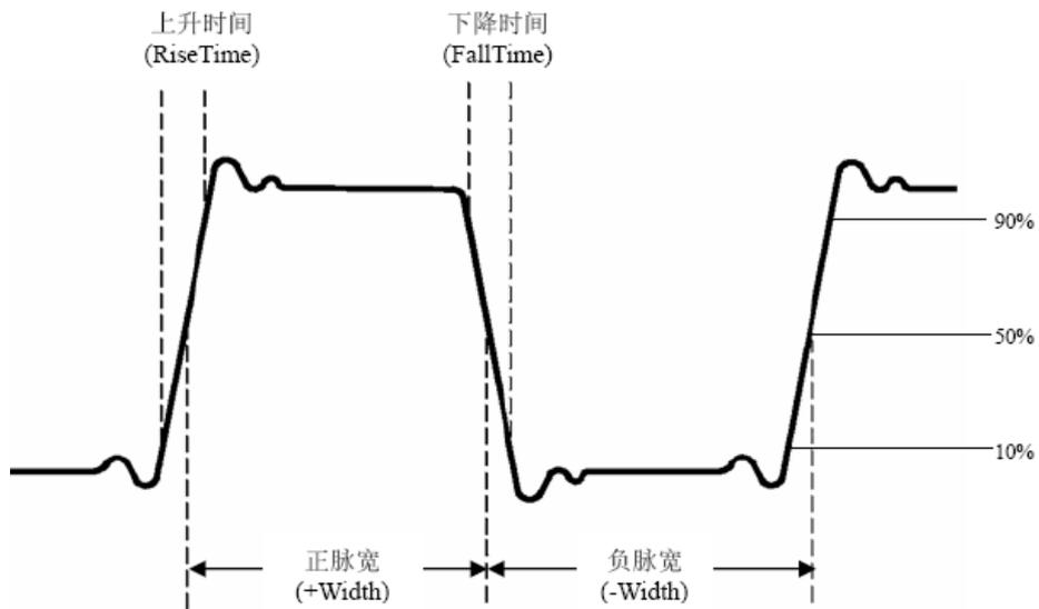
**RiseTime:** The time span for signal amplitude rise from 10% to 90%, judged by the rising edge of its first pulse.
